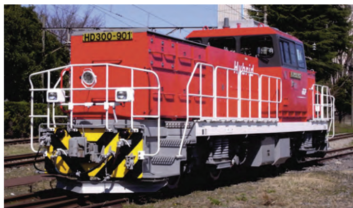
Fig. 1. Prototype of the Toshiba HD300 shunting locomotive [2]
