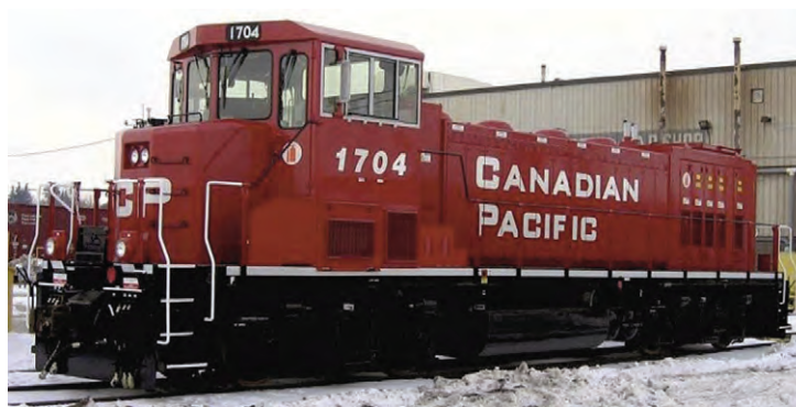
Fig. 5. The Railpower GG20B Green Goat shunting locomotive operated by Canadian Pacific [6]
