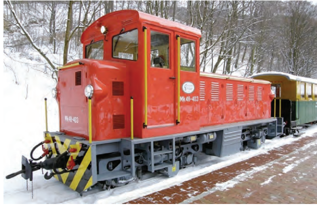
Fig. 11. Szilvássvár Forest Railway Rába Mk 48 battery-hybrid locomotive [16]
