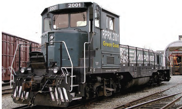
Fig. 4. The Railpower GGS2000D – a prototype of the GG20B Green Goat locomotive [6]
