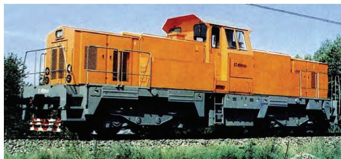
Fig. 10. The Řada 718 locomotive hybrid locomotive [15]
