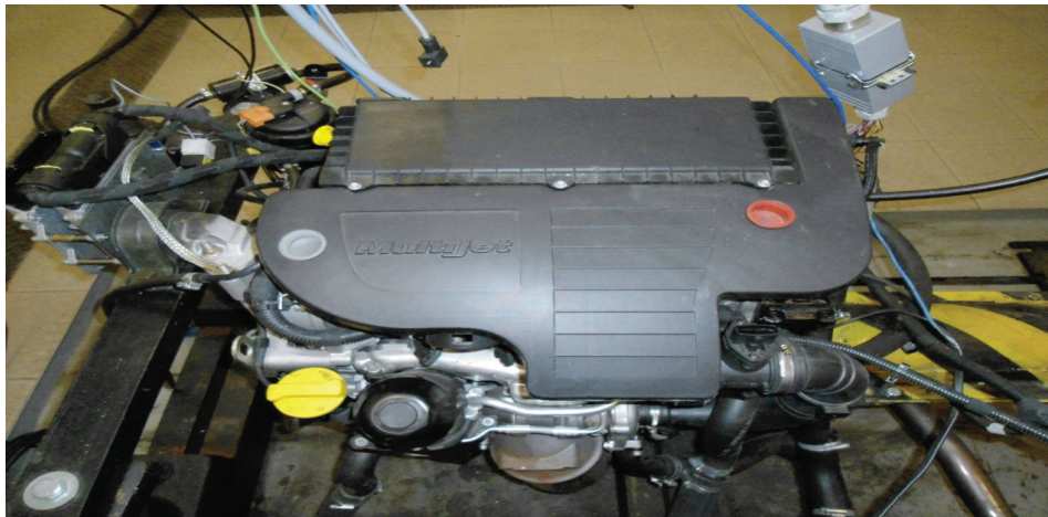
Fig. 1. FIAT Multijet 1.3 JTD 16 V engine with air filter being fitted
