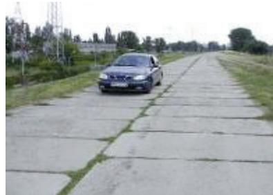
*Fig. 2. Test road section with “rough” surface*
