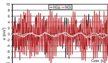
Fig. 7. Time histories of the head accelerations: test drives on the road section with “rough” surface (Br, cases NGp and NGt)
