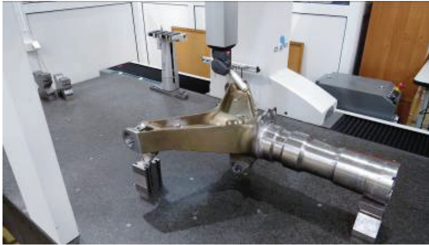
Fig. 4. Taking measurements on the Coordinate Measure Machine
