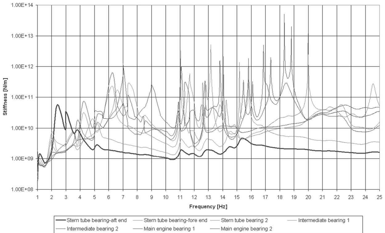
Fig. 3. The stern tube bearing's hull stiffness distribution
