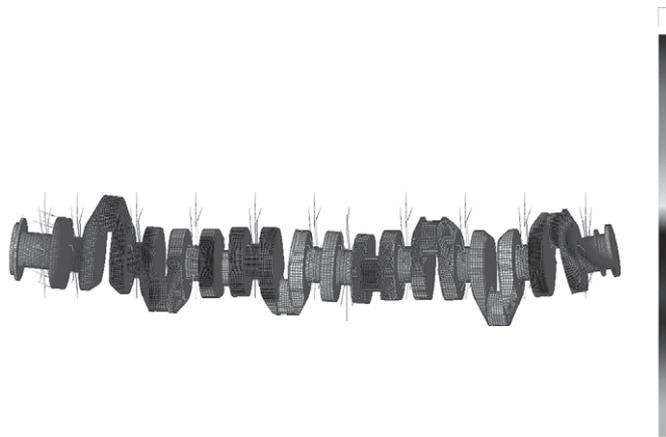
Fig. 5. Crankshaft deformation for elastic foundation
