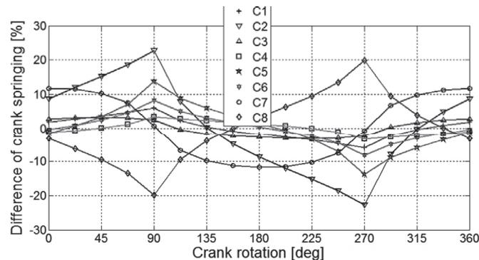
Fig. 6. Influence of foundation elasticity on crank springing
