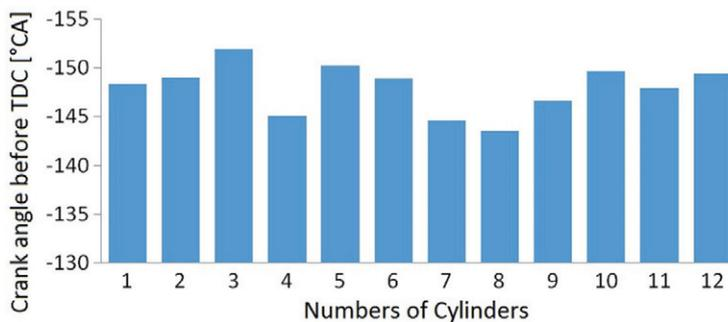
Fig. 9. Values of intake valves angles closing for auxiliary diese-generator engine WOLA H12; engine speed = 1500 rpm, engine load = 100% of nominal load
