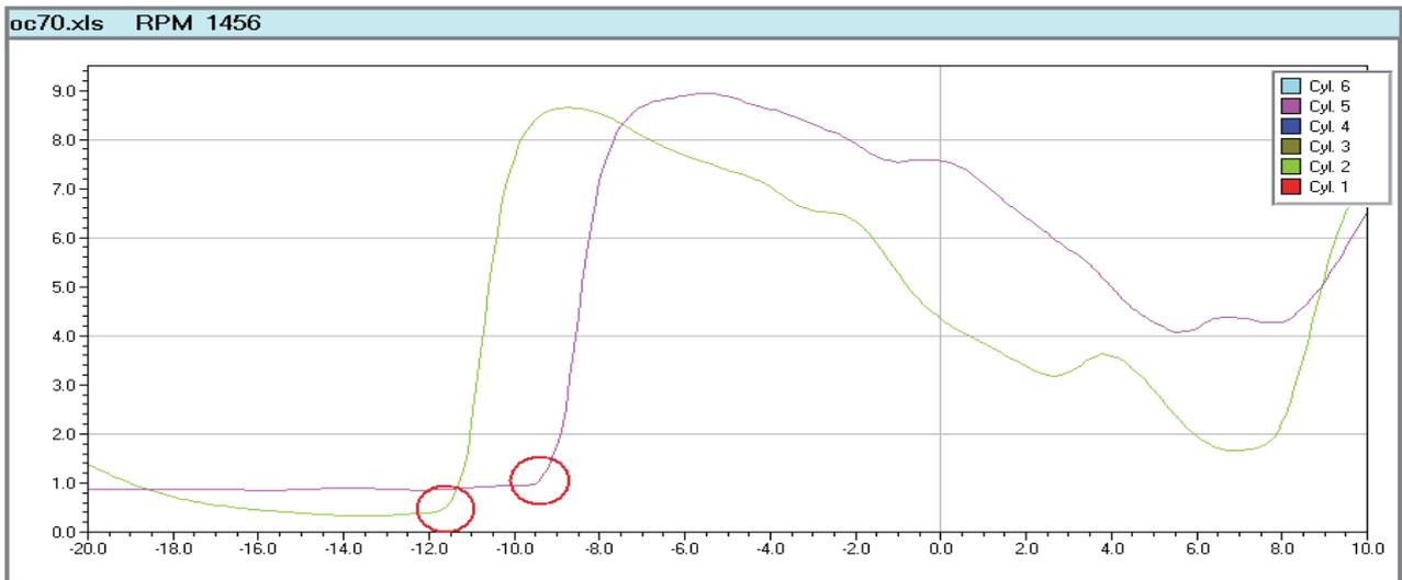
Fig. 5. Envelopes of vibration acceleration signals registered on the laboratory six cylinders diesel engine WOLA type 57H6Aa in „zoom“ mode circles – angles of fuel valves opens; engine speed = 1456 rpm, engine load = 34 kW = 25% of nominal load
