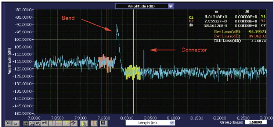
Fig. 4. Example signal from Luna optical backscatter reflectometer
