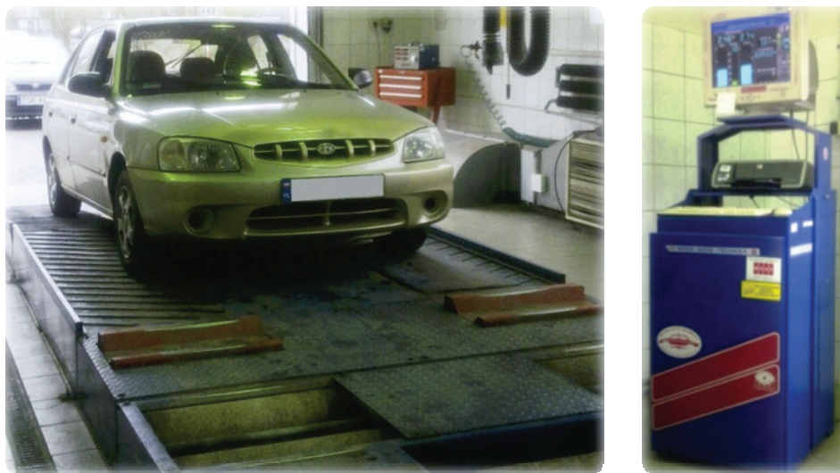
Fig. 1. Diagnostic stand with being tested Hyundai Accent II
