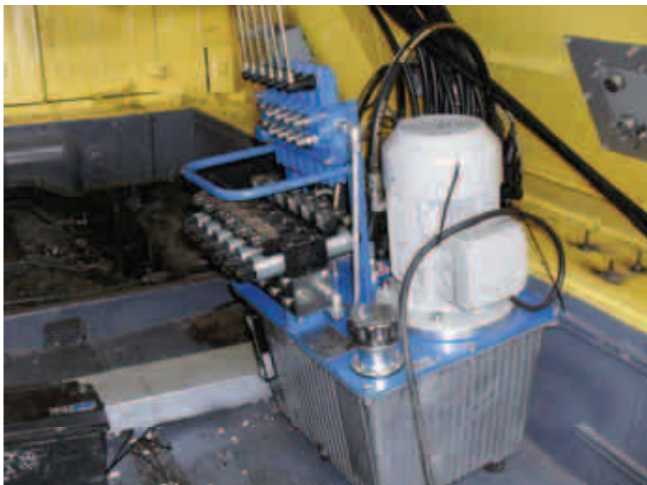
Fig. 4. Hydraulic pump mounted inside the vehicle
