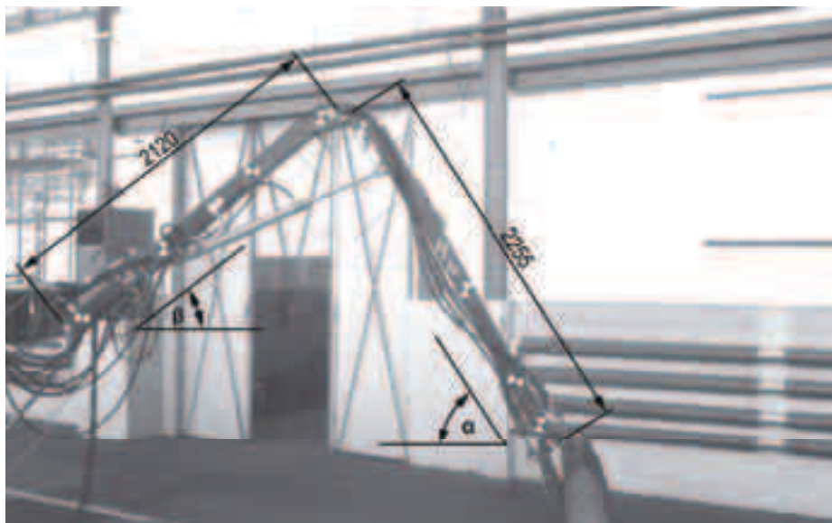
Fig. 2. Interrogation arm with specific dimensions and angle definitions
