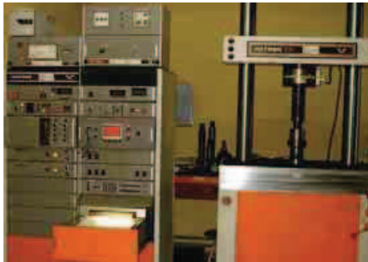
Fig. 1. Endurance machine static-dynamic of type Instron 1273
