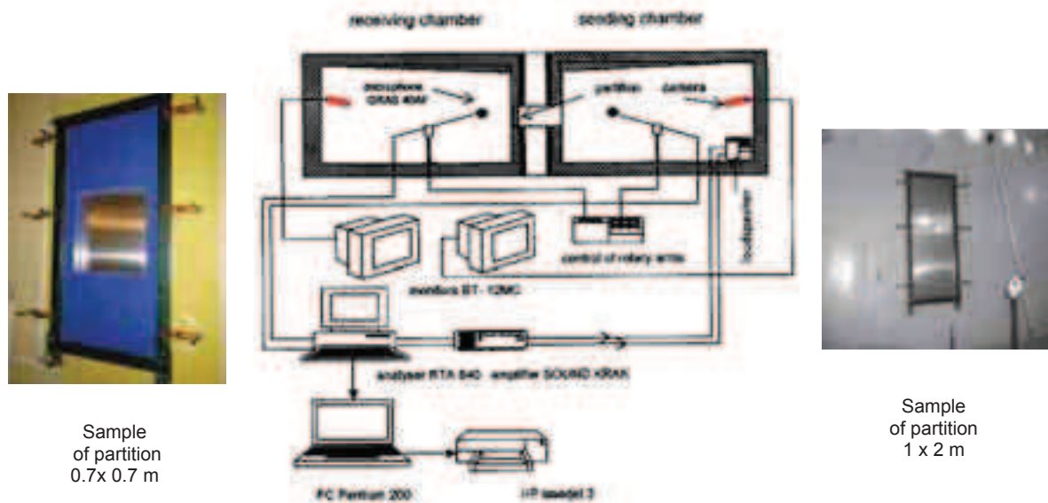
Fig. 7. Outline of the measuring path for measurements of the acoustic insularity appropriate of barriers applied in securities vibroacoustics
