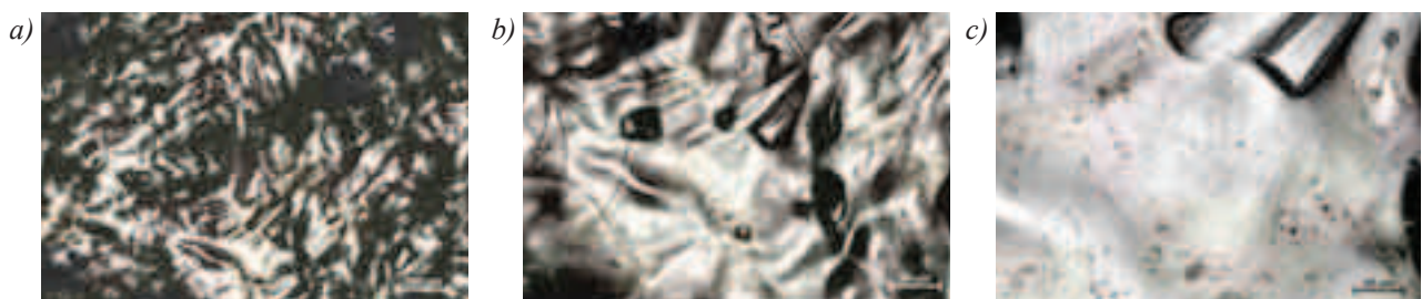
Fig. 2. MM images of 1 (CuZnNi) sample surface: a) the scale of 100μm, b) the scale of 50μm, c) the scale of 20μm
