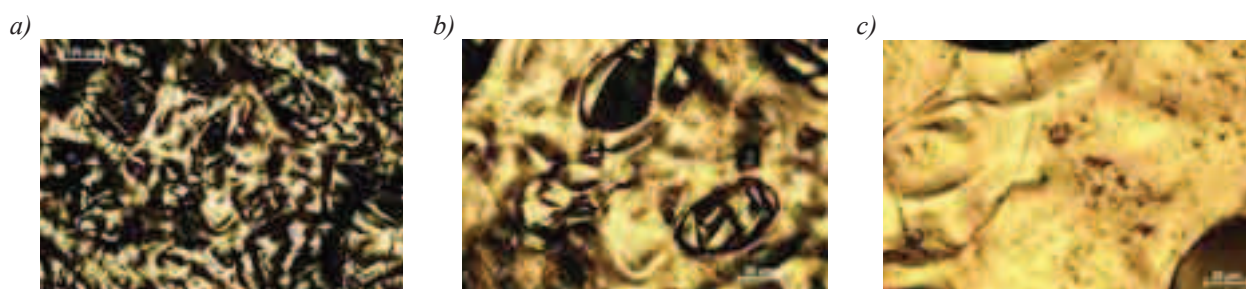
Fig. 5. MM images of 4 (three-layer system: CuZnNi / NiCuFe / CuSn) sample surface a) the scale of 100μm, b) the scale of 50μm, c) the scale of 20μm
