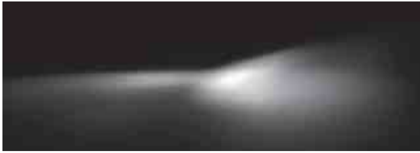
Fig. 2. Visualization of illuminance distribution of real headlamp beam pattern on vertical measuring screen corresponding type approval assessment
