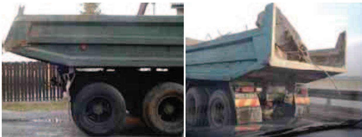
Fig. 14. The examples of protruding of bodies of the self-unloading trucks
