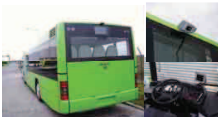
Fig. 11. The view of the bus, the placement of the camera and the screen of the projector in the cab
