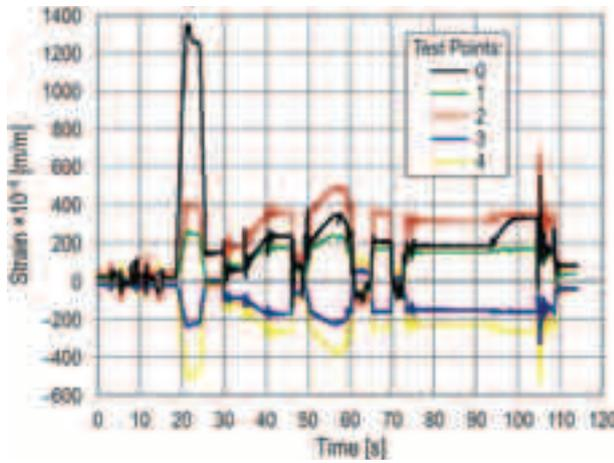
Fig. 6. Plots of the  $\epsilon$ - $t$  for test points 0–4
