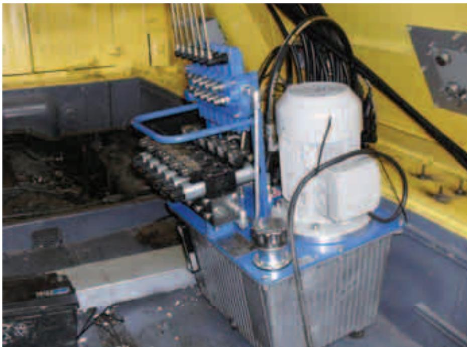
Fig. 4. Hydraulic pump mounted inside the vehicle
