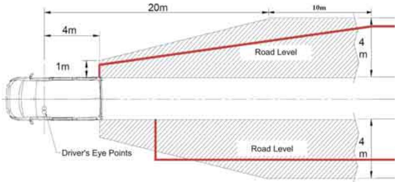
Fig. 3. Placement and vastness of the visibility field for the main rear view mirrors of class III – by thickened line denotes requirements hitherto in force -  $dmc \geq 2000$  kg [3]
