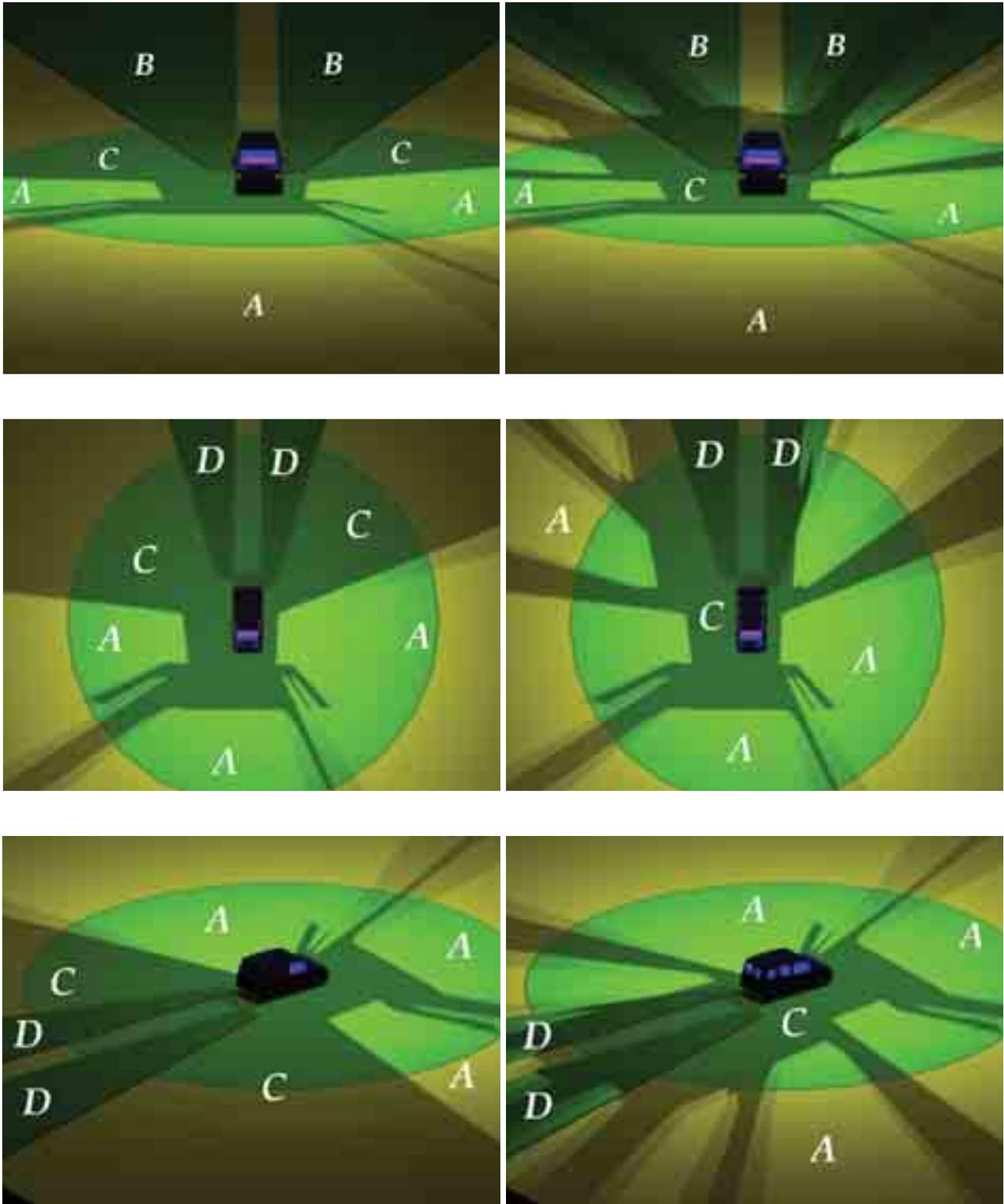
Fig. 5. The direct and indirect visibility field for – Renault Kangoo truck category N<sub>1</sub> and car category M<sub>1</sub>
