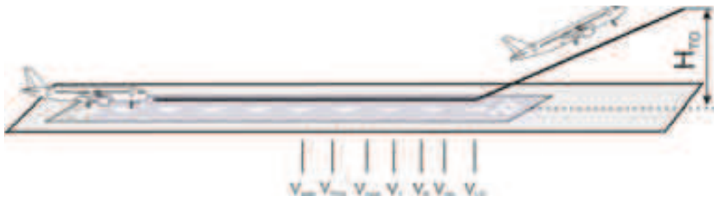
Fig. 1. Conventional take-off [4]. V_{STALL} - stall speed or the minimum steady flight speed at which the aeroplane is controllable, V_{MCG} - minimum control speed, on or near ground, V_{MCA} - minimum control speed, take-off climb, V_1 - critical engine failure speed, V_R - rotation speed, V_{MU} - minimum unstick speed, V_{LOF} - liftoff speed
