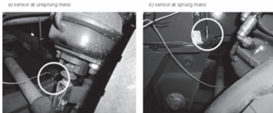
Fig. 2. Positioning of the accelerometers at the trailer suspension
