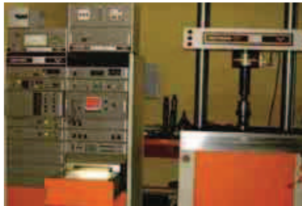
Fig. 7. Endurance machine static-dynamic of type Instron 1273
