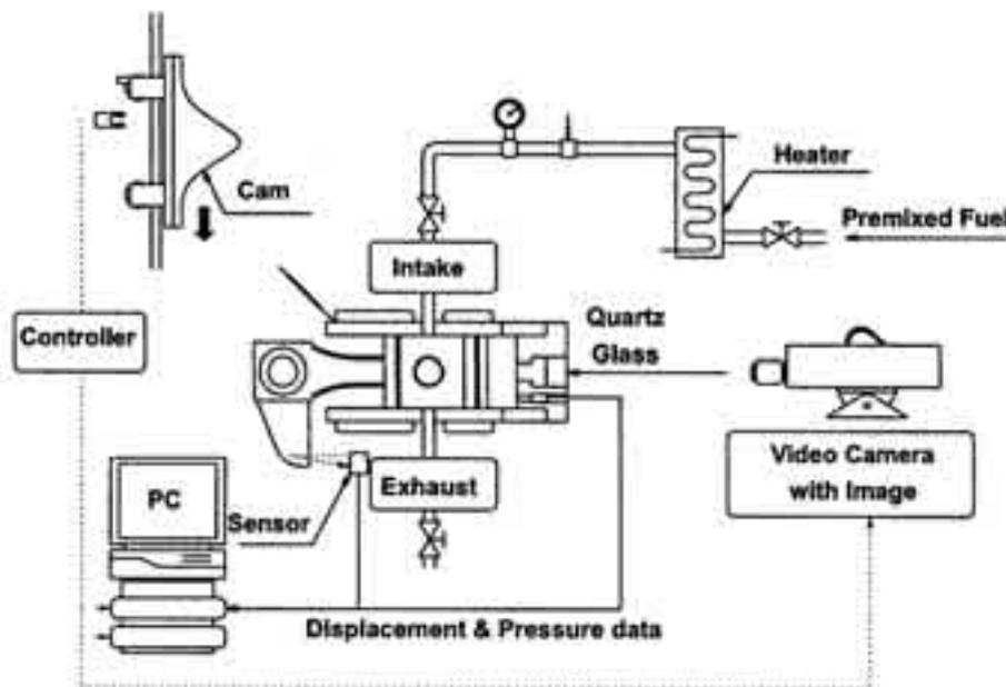
Fig. 7. Schematically presented RCM of pneumatically driven with doublet cam [1]
