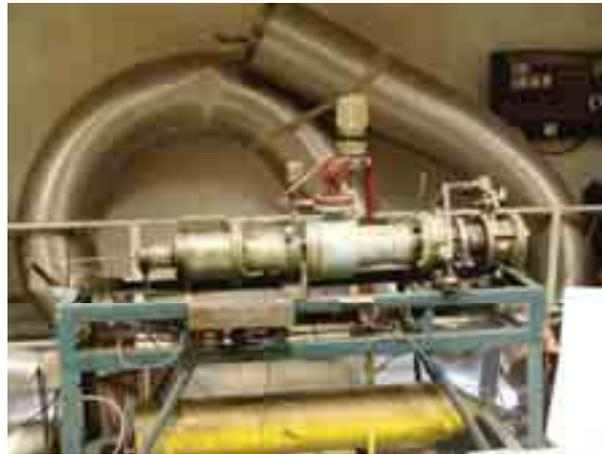
*Fig.2. View of pneumatically driven RCM*
