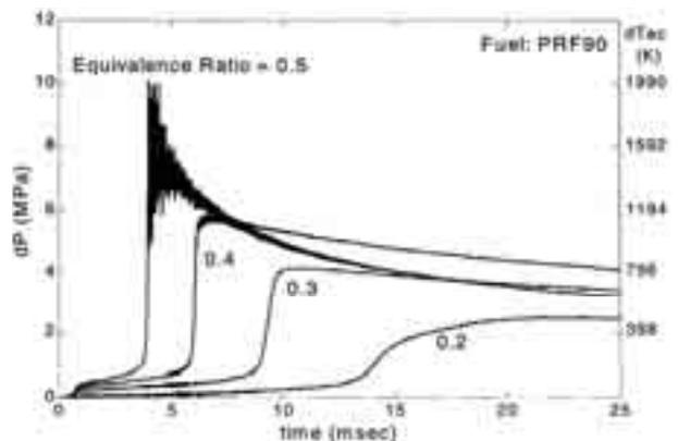
Fig. 12. Effect of equivalent ratio on ignition delay [4]
