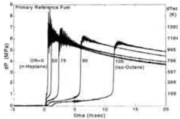
Fig. 11. Effect of octane number on ignition delay [4]
