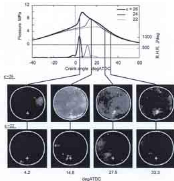
*Fig. 9. Effect of compression ratio on HCCI combustion [1]*
