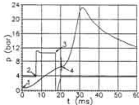
Fig. 3. Example of the high-speed pressure histories
