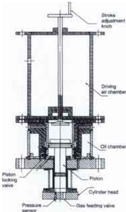
Fig. 10. Schematic of RCM from MIT [4]
