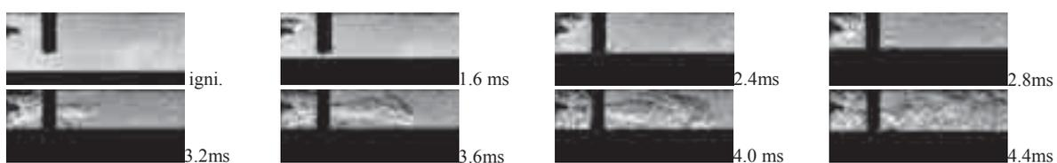
Fig. 6. The combustion development in the new combustion system : ignition advance angle 35° CA BTDC
