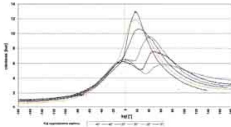
Fig. 8. The waveforms of pressure in the combustion chamber versus crankshaft rotation angle for different values of ignition advance angle
