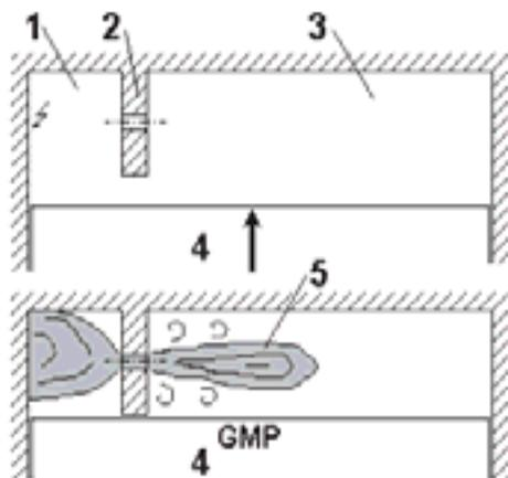
*at ignition the prechamber and the main combustion chamber are filled up with homogeneous, stoichiometric mixture and they are open*
