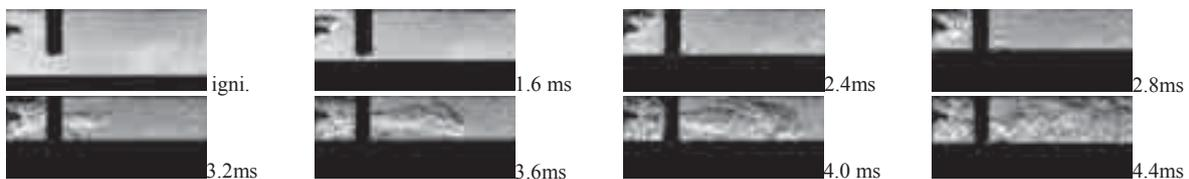
Fig. 6. The combustion development in the new combustion system : ignition advance angle 35° CA BTDC
