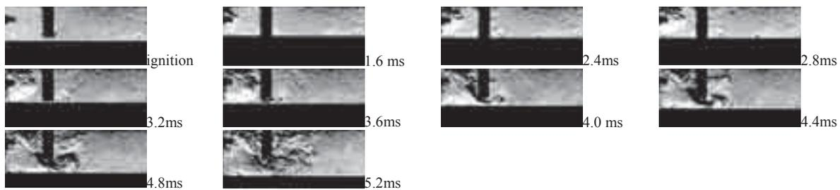
Fig. 9. The combustion development in the new combustion system : ignition advance angle  $20^{\circ}$  CA BTDC
