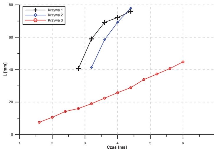
Fig. 7. The comparison of the stream front displacement for ignition advance angle  $20^{\circ}$  and  $35^{\circ}$  CA BTDC
