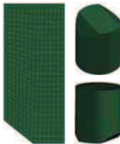
Fig. 5. The simplified numerical model of the 20 mm 54 g FSP standard fragment
