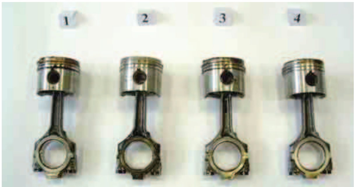
Fig. 7. The view of the piston groups after the tests
