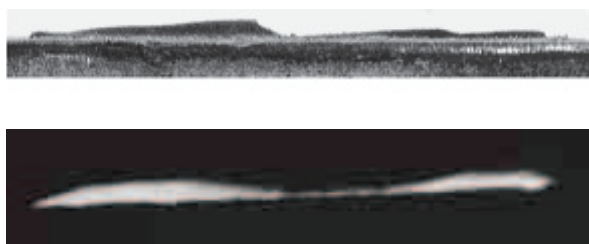
Fig. 5. Cross-section of burnt stripe of solid fuel in comparison to cross-section of the thermal boundary layer for burnt fuel stripe
