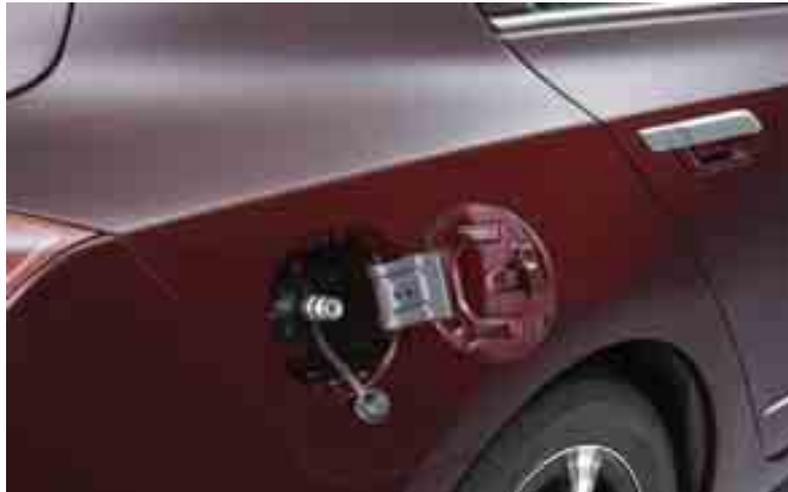
*Fig.1. Honda's FCX Clarity hydrogen tank inlet*
