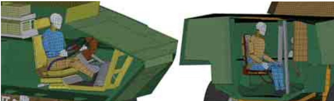
Fig. 1. The location of dummies inside a carrier: driver (left), crew member (right)
