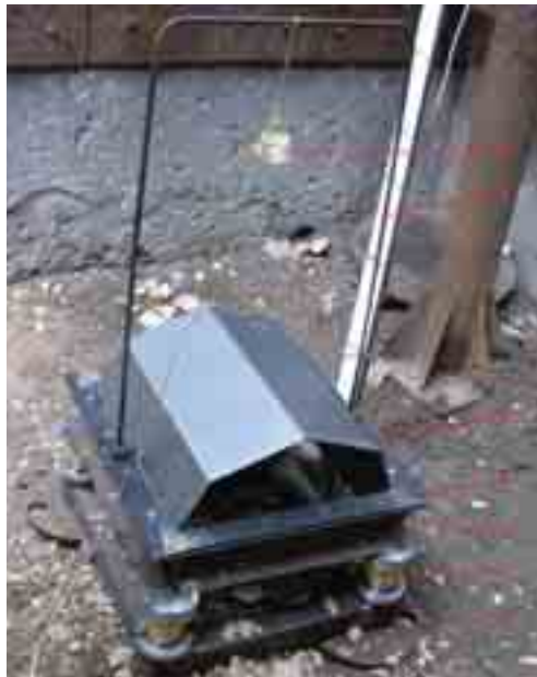
Fig. 2. Test stand used in experimental research: 1 – base, 2 – strain gauge force transducer (4 pieces), 3 – mounting frame, 4 – upper mounting frame, 5 – deflector, 6 – explosive charge mount, 7 – explosive charge
