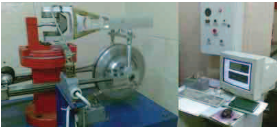
Fig. 2. The laboratory fatigue testing of materials
