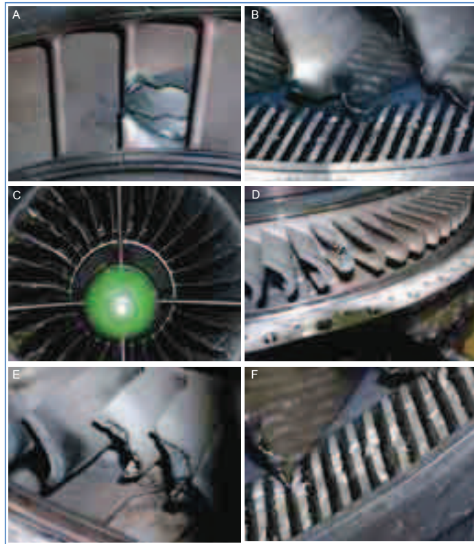
Fig. 2. Characteristic damage of RD-33 engines
