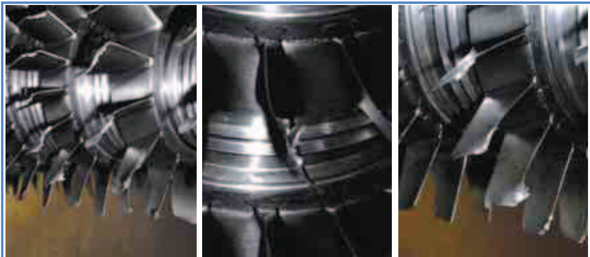
Fig. 1. Characteristic damage of GTD-350 engines
