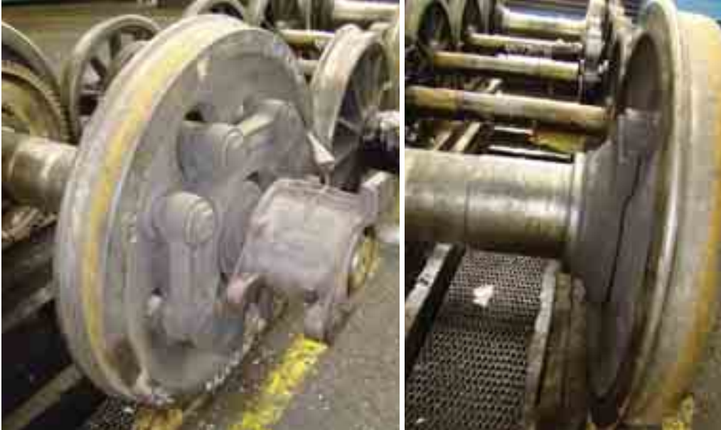
Fig. 1. The dismantled axes from diesel shunting locomotives SM42
