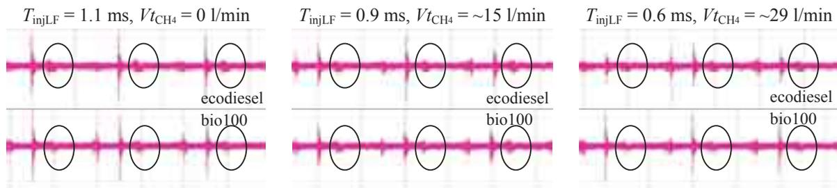
Fig. 4. Fragments of timing diagrams for vibration signals registered on the body of HATZ 1B40 engine for a set rotational speed of the crankshaft of 3000 rpm when the engine is fed with various air-fuel mixtures; marked oval fragments reflect the liquid fuel injection, its self-combustion and the onset of air-fuel mixture combustion
