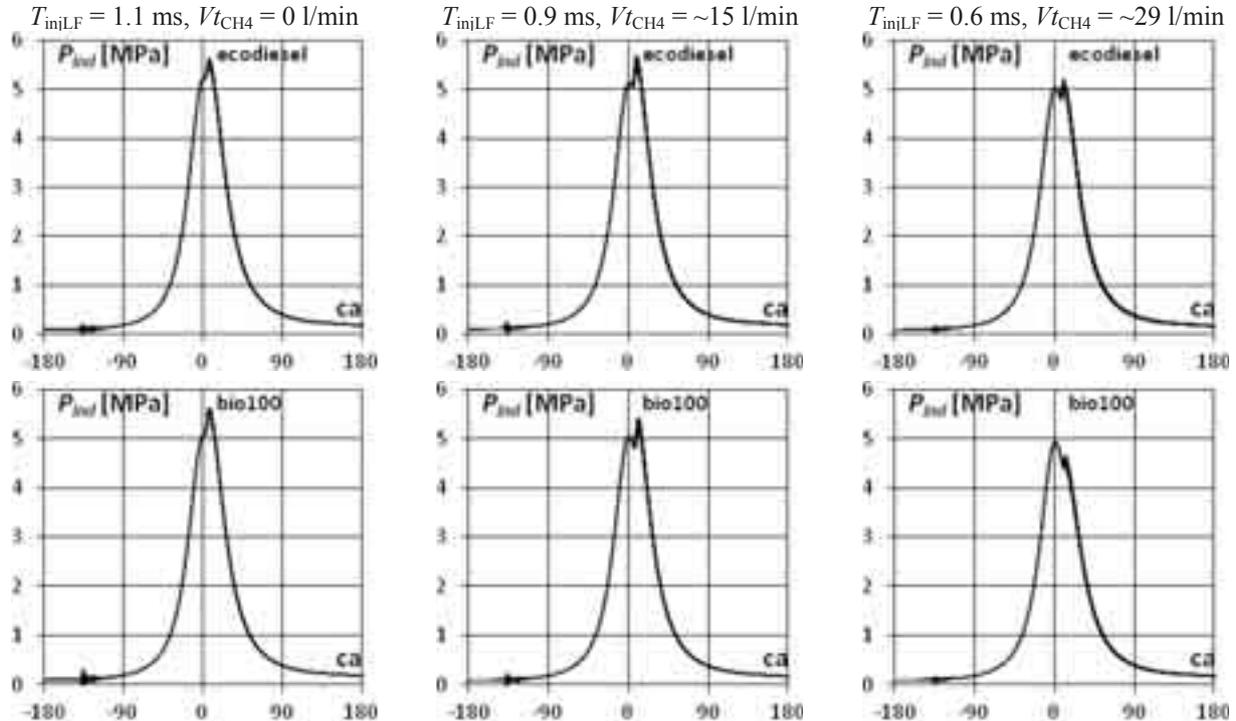
Fig. 2. Changes of pressure  $P_{ind}$  in the cylinder of the analysed engine fed with various air-fuel mixtures (20 fragments of engine performance cycles lining up)
