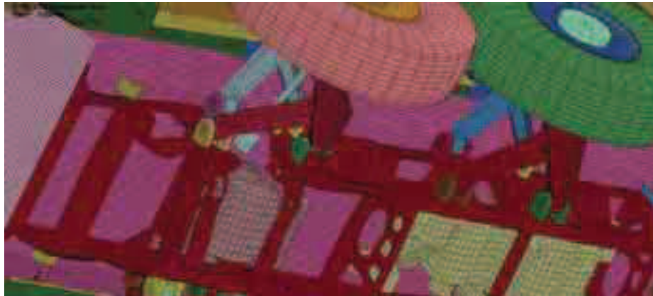
Fig. 19. Damages of indirect support and a vehicle body resulting from an explosion of a 25 kg TNT explosive
