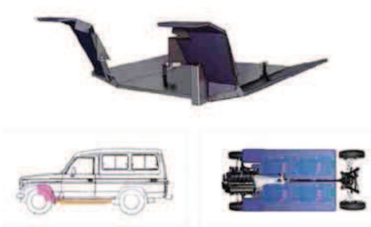
Fig. 10. Shape and arrangement of additional protection elements before the explosion of mines and IED [Aigis Blast Protection Ltd UK]
