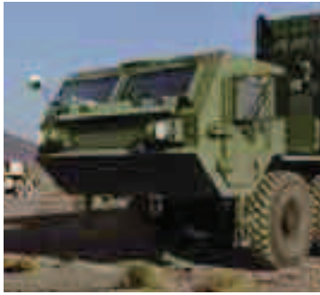
Fig. 7. Oshkosh A4 HEMTT – heavy tactical vehicle with increased mobility "B kit" shield [13]
