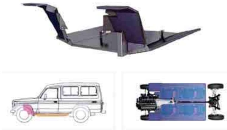
Fig. 10. Shape and arrangement of additional protection elements before the explosion of mines and IED [Aegis Blast Protection Ltd UK]
