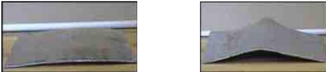
Fig. 9. A plate made of TABREarmour® material before and after the tests [Aegis Blast Protection Ltd UK]
