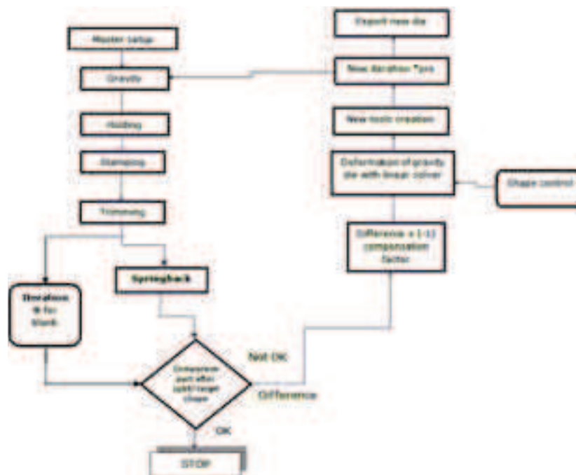
Fig. 2. Process of die compensation [9]
