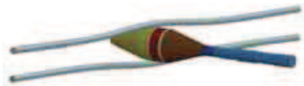
Fig. 15. Numerical analysis of projectile impact into rods – the initial stage
