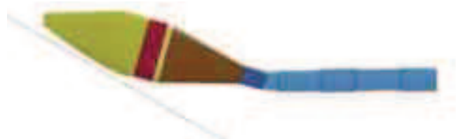
Fig. 9. Impact into the plate - the projectile rear part is fully disconnected
