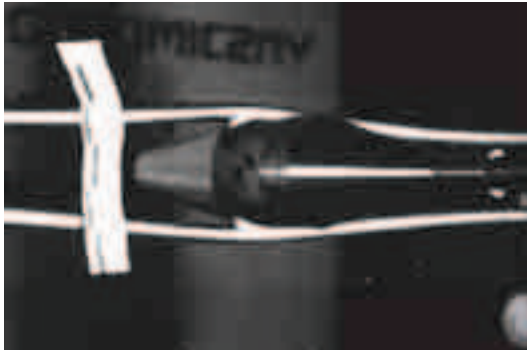
Fig. 13. Projectile impact into steel rods –the initial stage of the process
