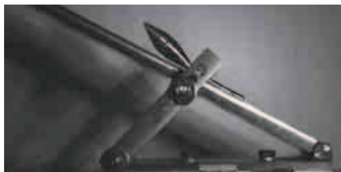
Fig. 7. Impact into the plate – the shank hits into the plate
