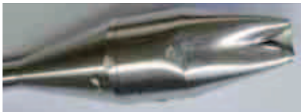
Fig. 11. Front part of the projectile after impact into the rod
