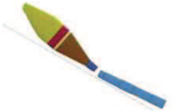
Fig. 10. Impact into the plate – the shank hits into the plate
