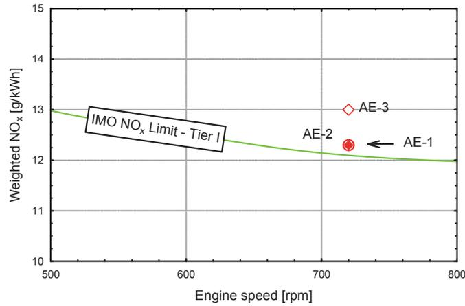
Fig. 7. NOx emission factors for ship diesel engine generators in Tier 1 limit
