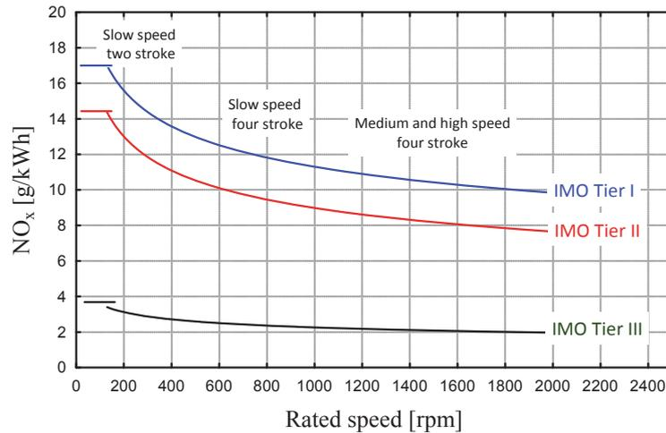
Fig. 1. Nitrogen oxides emission limits for marine engines
