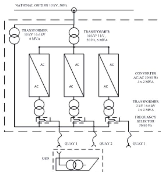
Fig. 3. The "Shore To Ship" concept for ferry terminals
