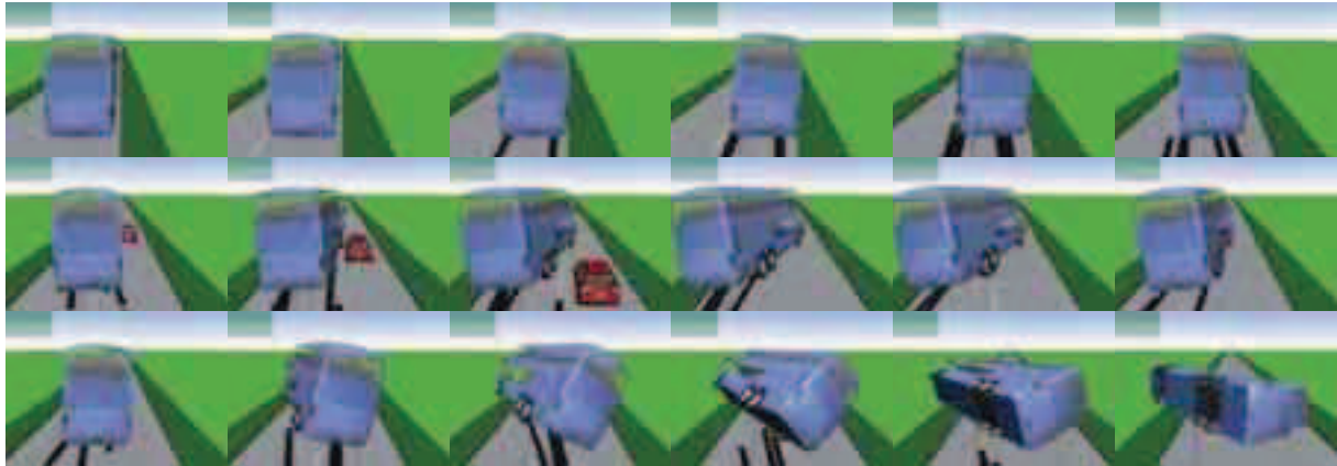
Fig. 4.1. An example of the results (a sequence of pictures) of a simulation of the bus rollover process at the avoidance of an obstacle having suddenly sprung up; bus without passengers, driven with a speed of 110 km/h
