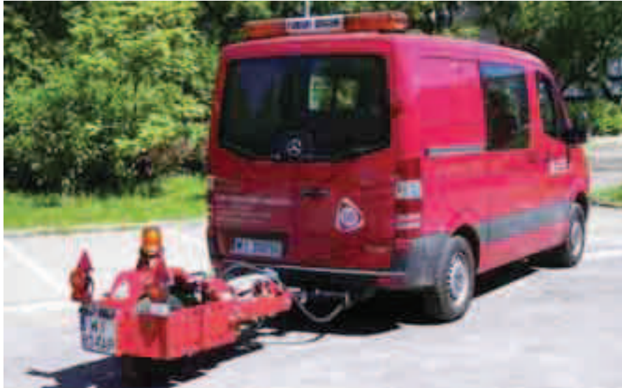
Fig. 1. Measurement system SRT-4 – Mercedes-Benz Sprinter and dynamometer trailer
