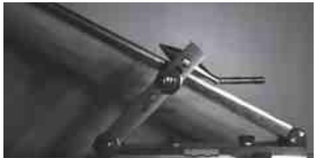
Fig. 5. Impact into the plate - beginning of bending of the projectile rear part
