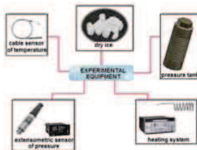
Fig. 5. Research equipment for CO 2 thermodynamic behaviour testing
