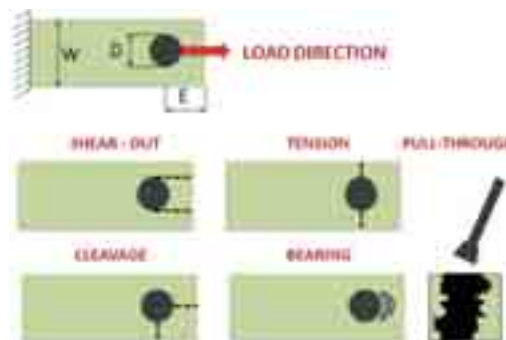
Fig. 5. Failure mechanism in bolted composites [3]
