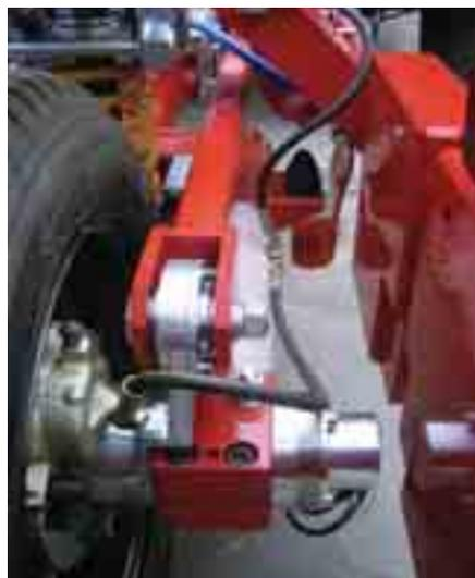
Fig. 2. Measurement wheel of dynamometer trailer
