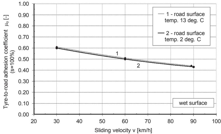
Fig.5. Velocity characteristics  $\mu_0(v)$  for different ambient temperatures
