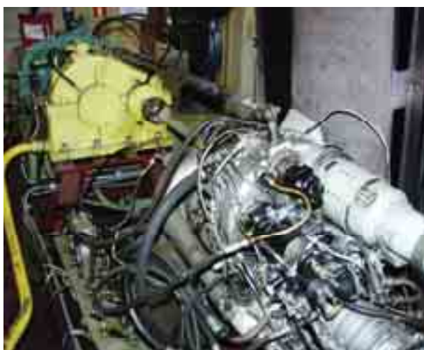
Fig. 1. The laboratory stand with the gas turbine engine GTD – 350
