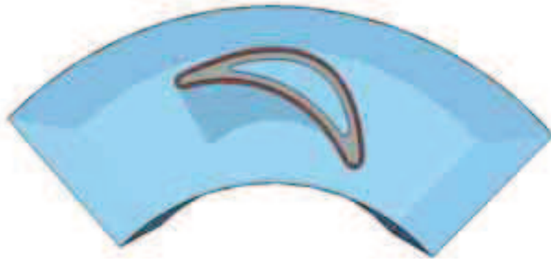
Fig. 2. Blade and surrounding gas canal
