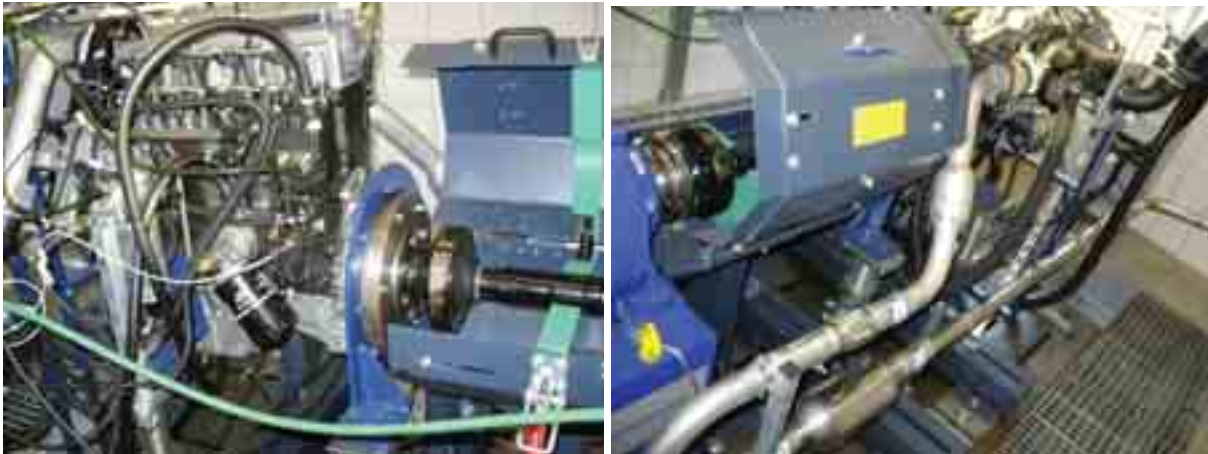
Fig.3. The ADCR engine on the test bed; The exhaust train of the ADCR engine mounted on the test bed
