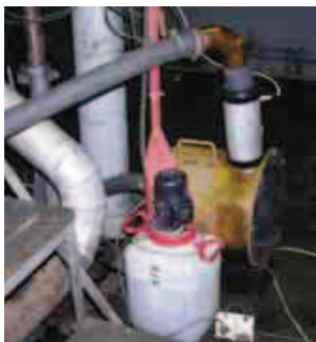
Fig. 7. The equipment of the research stand to measurement of blowthrough to the crank case
