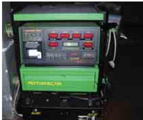
Fig. 8. The equipment of the research stand – exhaust emission analyzer
