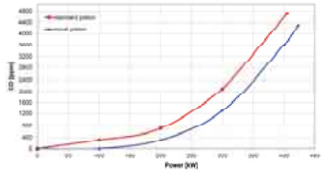
Fig. 21. Courses of the concentration of the carbon monoxide (CO) for the part load characteristics 1200 rpm
