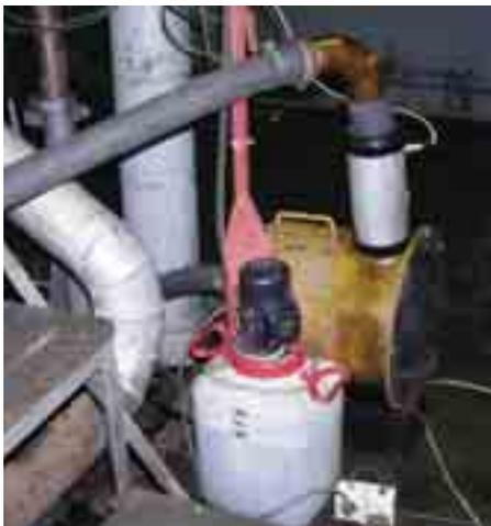
Fig. 7. The equipment of the research stand to measurement of blowthrough to the crank case
