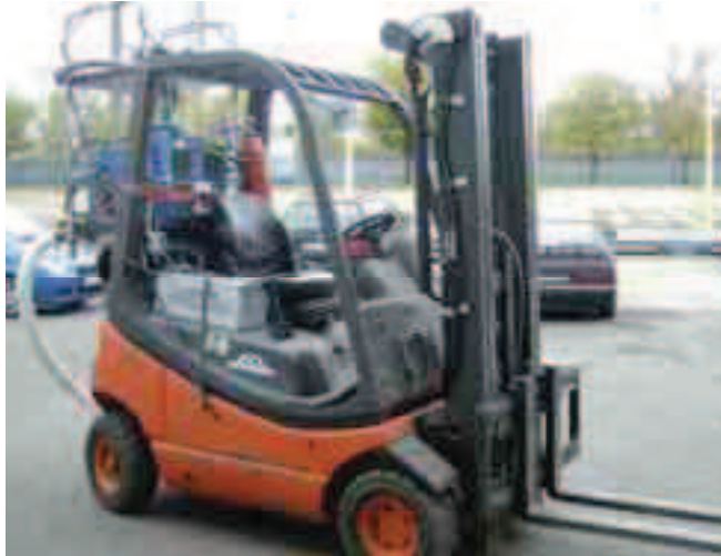
Fig. 1. The forklift truck with the equipment installed for the measurement of gaseous pollutants emissions in the real conditions
