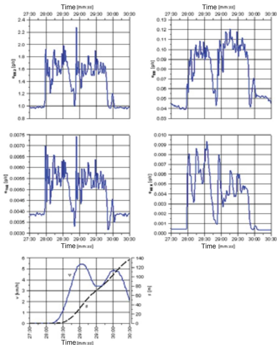
Fig. 4. Change in emission intensity of selected exhaust components emitted from a forklift truck moving during operation; run No. 6
