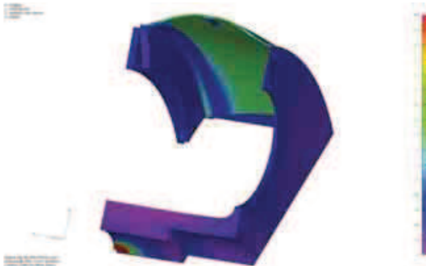
Fig. 6. Reduced stress levels in barrel computational model at 10000 rpm with additional mass
