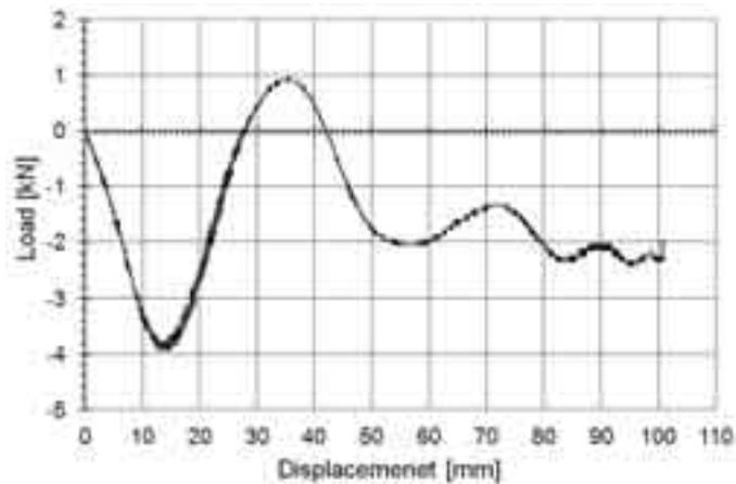
Fig. 8. Dependence of spring load on beam displacement
