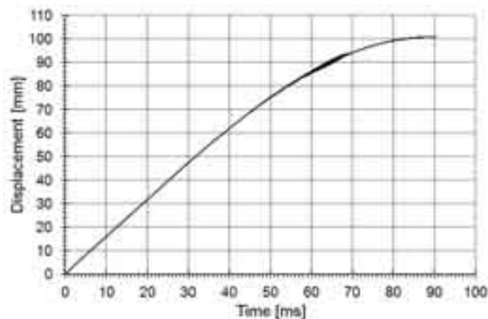
Fig. 9. Displacement of hammer beam loading spring
